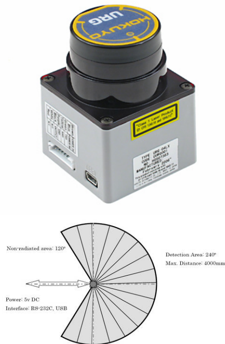
Fig. 7. Laser sensor (Hokuyo URG-04LX) and its field of view
