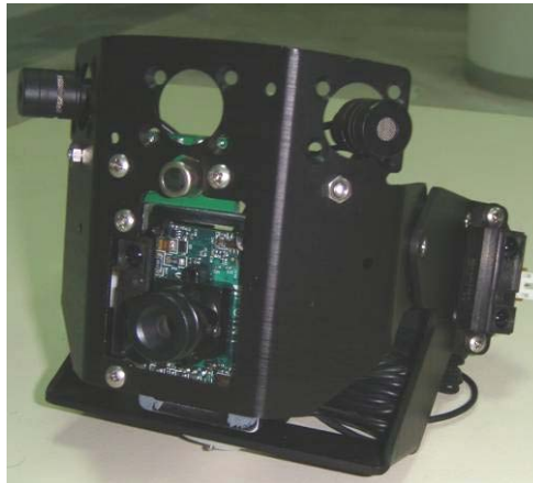
Fig. 15. Camera Head mounted on a robotic arm without the CO 2 sensor
