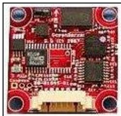
**Fig. 16.** Ocean Server OS5000 3 Dimensional Compass
