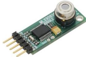
**Fig. 11.** The MLX90614 Infrared Thermometer
